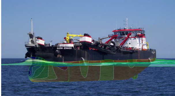
Fig.5: Hull optimization for a dredger
