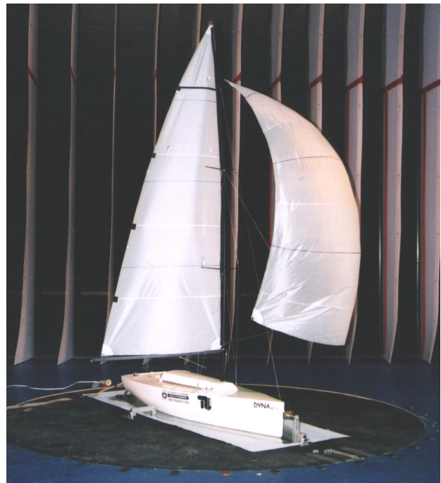
Figure 2. Model with mainsail and spinnaker in the TFWT
