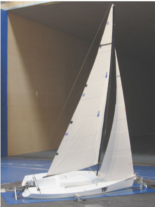
Figure 5: Wind tunnel model of the 10-metre IMS cruiser/racer DYNA
