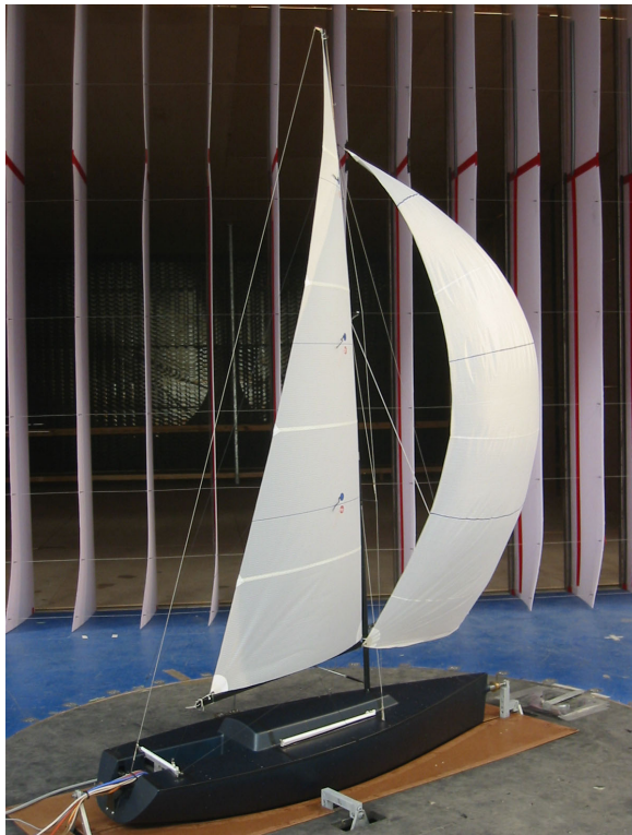
Figure 9 Scale model of a 10m IMS cruiser racer yacht in the Twisted Flow Wind Tunnel
