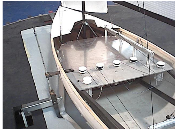
Figure 10 Inside of a wind tunnel model showing remote control winches to trim sails as in real life
