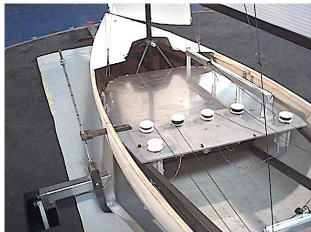
Figure 2: Inside of a wind tunnel model showing remote control winches and load carrying internal frame structure
