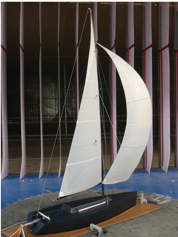
Figure 1: Scale model of a 10m IMS cruiser/racer yacht in the twisted flow wind tunnel
